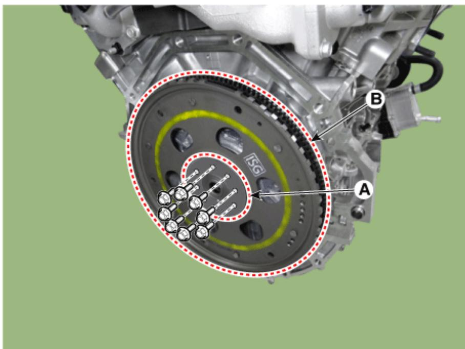
4. Remove the crankshaft adapter (A).
